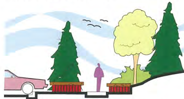
USE SCREEN WALLS, RAISED PLANTERS OR OTHER DEVICES TO PROTECT LANDSCAPING FROM PEDESTRIANS AND AUTOMOBILES.
